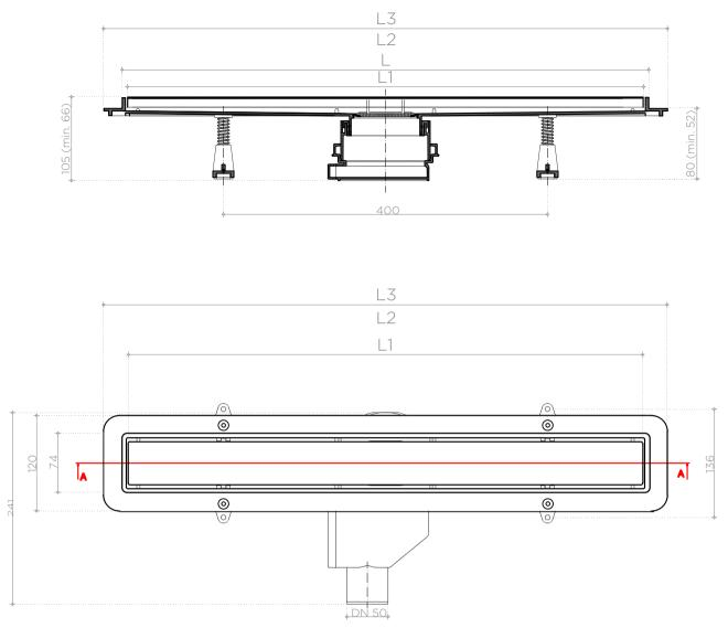
NOTE: Drains in length of 300, 450, 550 and 650 come in package with two sets of legs for adjusting of height. Drains in length 750 and 850 come in package with four sets of legs for adjusting of height.
